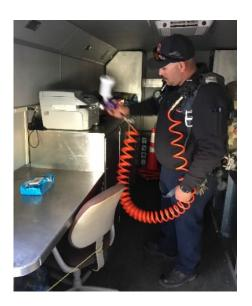
Photo illustrating SCBA Compressed Air System in use. Remember that all operators are required to wear ALL PPE during decontamination process: head wear, eye protection, face masks, gloves, disposable gown or body coverings.
