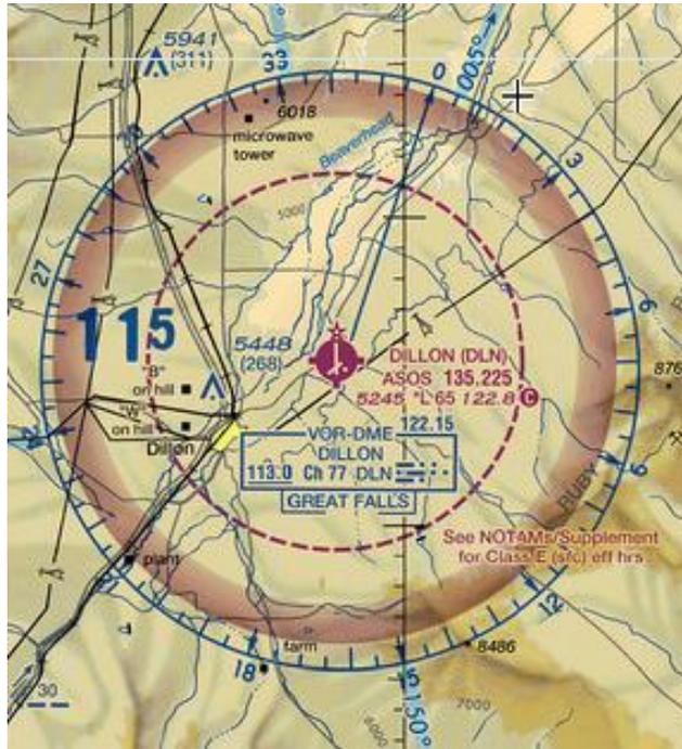
Figure 3-9: Class E Airspace Designated to the Surface by a Dashed Magenta Line
