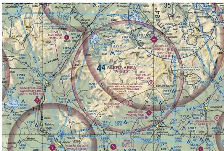
Figure 3-22: Alert Area Depicted on a Sectional Aeronautical Chart
