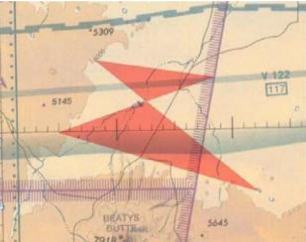
**Figure 6-8: TFR Coordinates Entered in Incorrect Clockwise Sequence**
