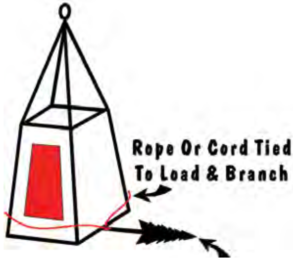
Exhibit 11-4: Rigging A Box-like load with a Tree Branch as a Tail
