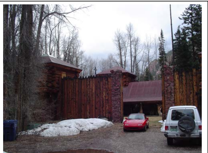
Large amounts of down/dead fuels are around the access route and the structure. These fuels need to be removed.
