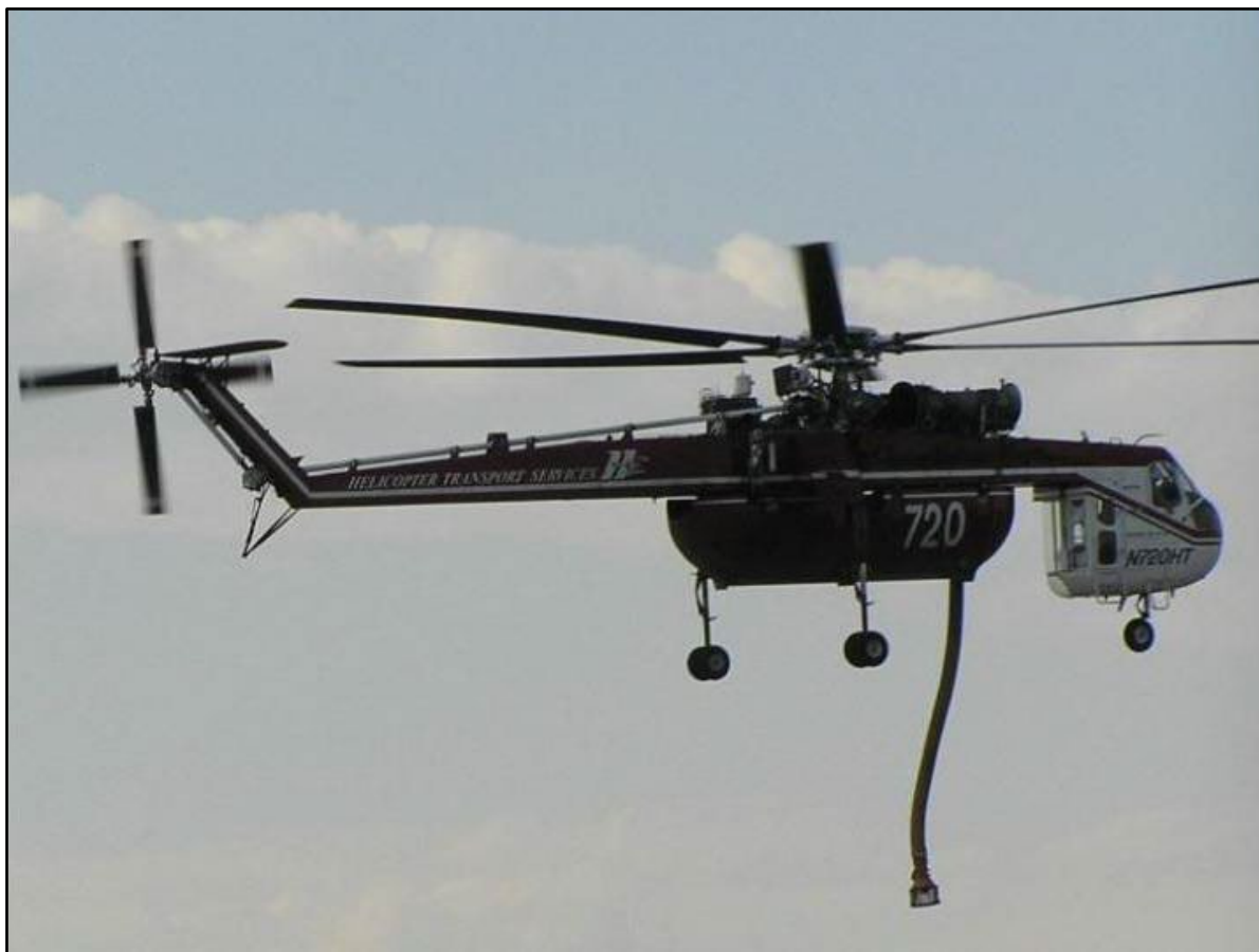
Sky Crane with Dipping Snorkel Assembly
