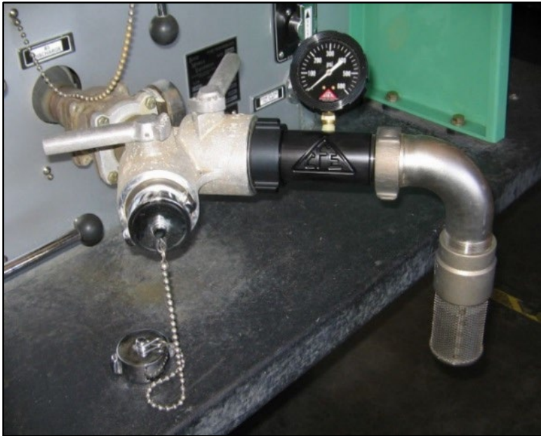
Foot valve attached to suction line with various adapters as needed to adjust for foot valve size.
