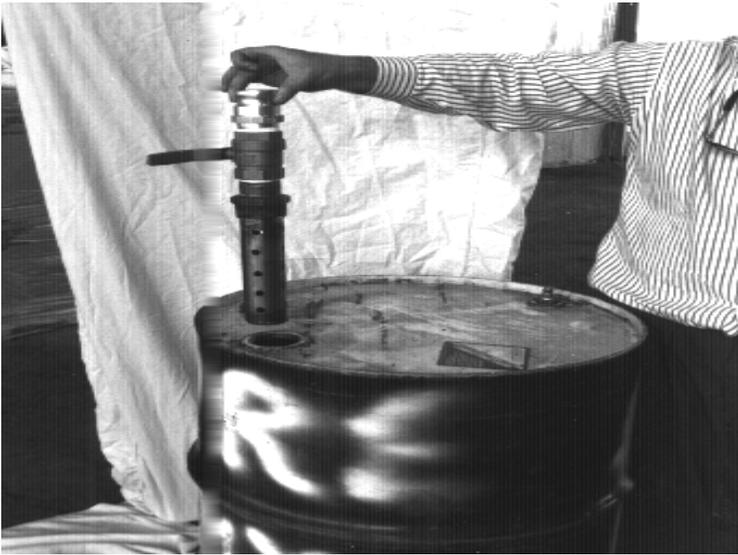
The Barrel Helitorch uses unmodified standard 55-gallon fuel drums. The ground crew must check the drums for fuel leaks and bent rims. Drums with bent rims on the vent bung side of the drum, or large dents in the side of the drum near drum rims, cannot be used since this is the area where the drum attaches to the helitorch. Any drum with damaged threads should not be used because it may leak or damage the threads of the helitorch vent or helitorch coupler.
