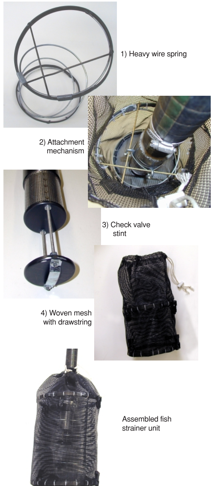
Figure 1—Fish strainer and components.
