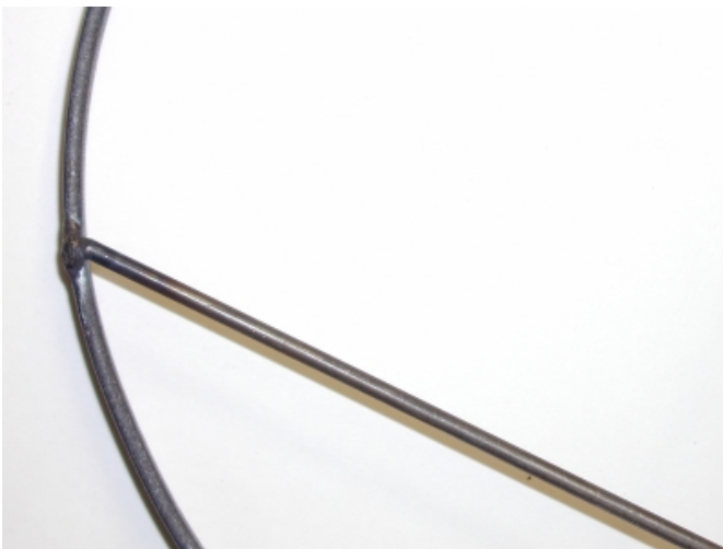
Figure B5—Place two layers of duct tape over wire or sharp edges.
