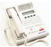
Vega C-2002 remote consoles are linked to a nearby Bendix/King base station (GBH model) and used to transmit/receive via the base station from an alternate location.
