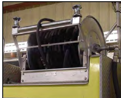
Engine hard line hose reel
