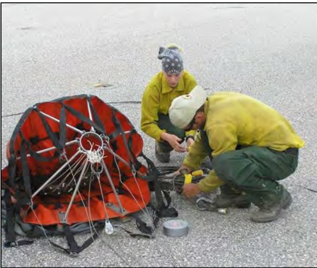
Crews working on an aerial "Bambi" bucket
