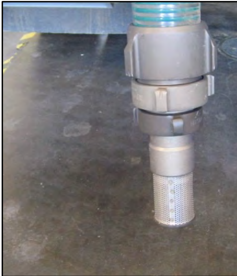
Foot valve attached to suction line with various adapters as needed to adjust for foot valve size.
