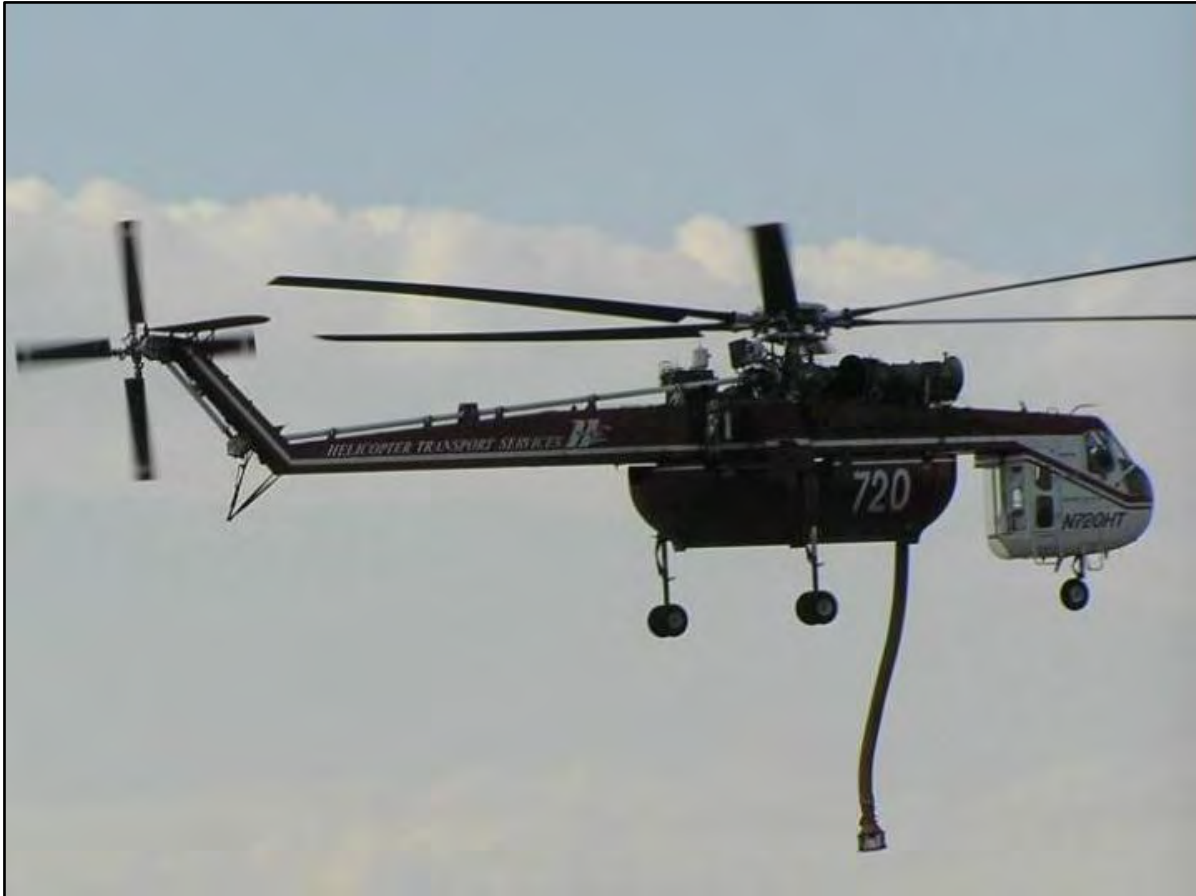
Sky Crane with Dipping Snorkel Assembly
