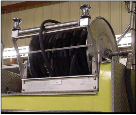
Engine Hard Line Hose Reel
