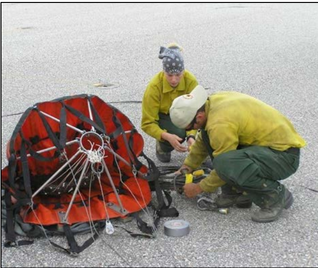
Crews working on an aerial "Bambi" bucket
