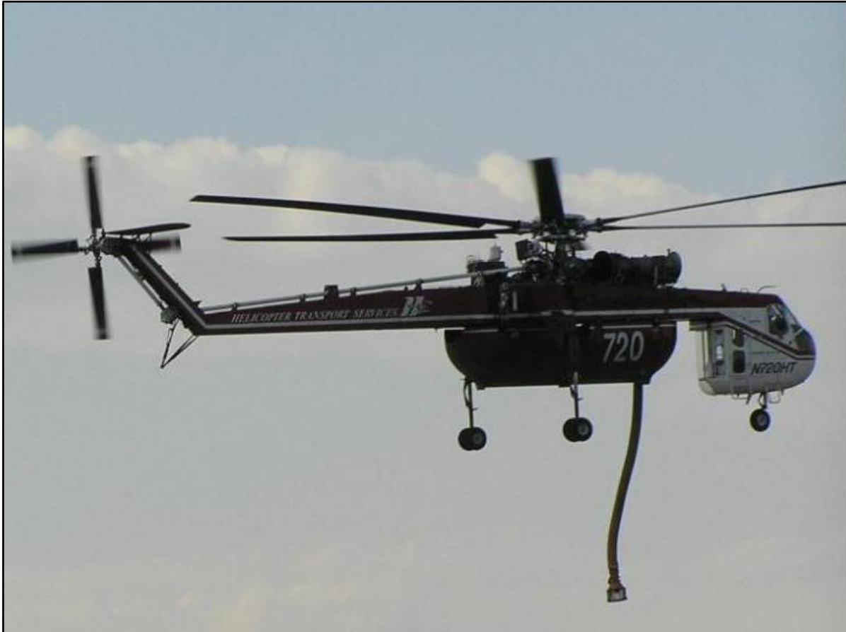
Sky Crane with Dipping Snorkel Assembly
