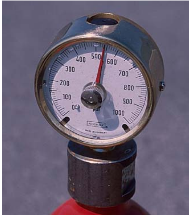
The pressure in this overfilled fuel bottle reached almost 550 psi before the bottle burst
