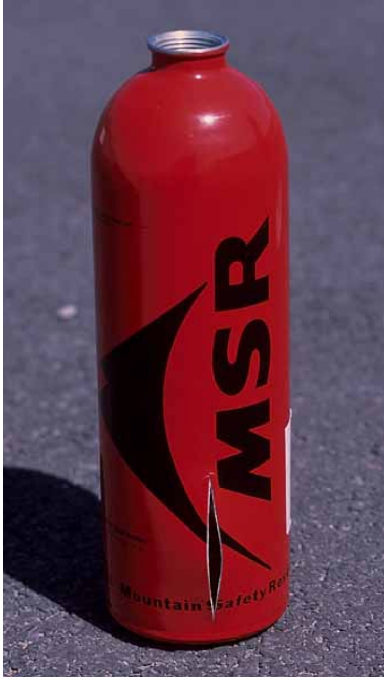
An example of a fuel bottle that burst from too much pressure
