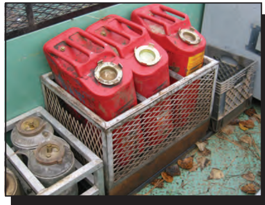
Figure 59—Fuel tanks for the Mark-3 pump secured properly for transport.
