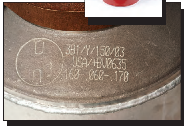
Figure 17—The UN marking shows that this drip torch meets DOT specifications.
