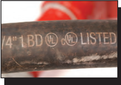
Figure 107—An example of an approved hose.
