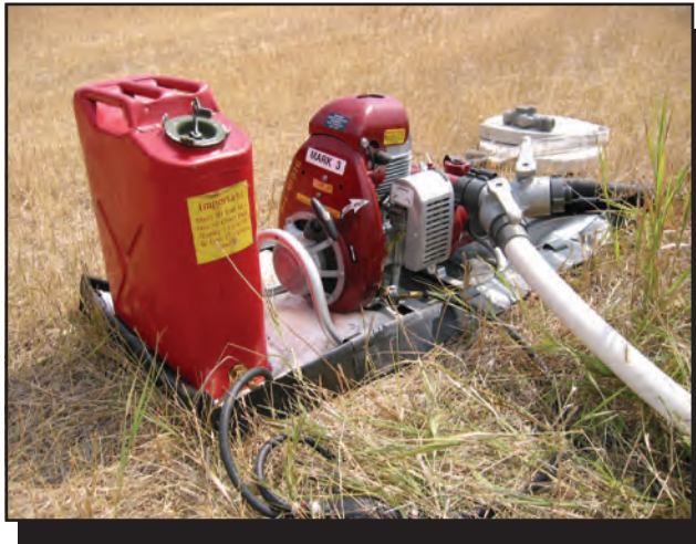
Figure 57—A fuel tank attached to a Mark-3 pump that is ready for operation.
