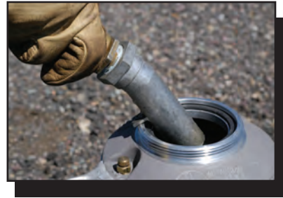
Figure 90—When a drip torch is filled properly, the pump nozzle touches the container, preventing sparks from static electricity generated by flowing fuel.
