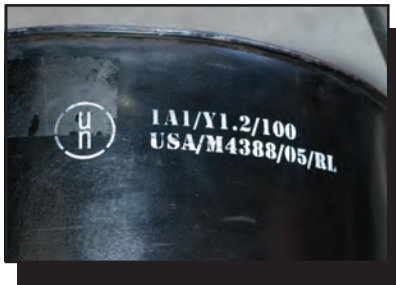
Figure 82—Approved drums have a UN number.
