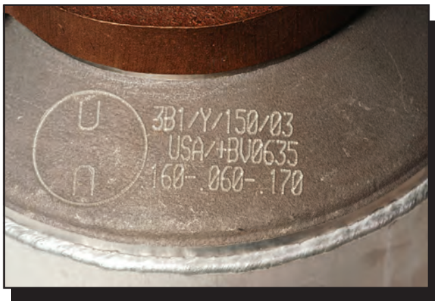
Figure 38—The UN marking shows that this drip torch meets DOT specifications.
