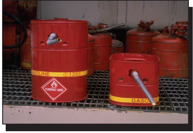
Figure 50—Safety transport cans showing the colors required by OSHA and the proper markings.
