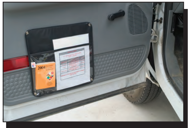
Figure 33—An example of an appropriate storage location for shipping papers and the Emergency Response Guidebook .
