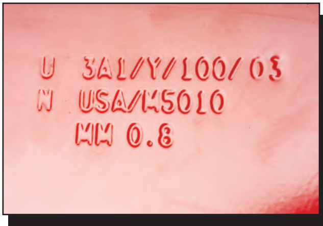
Figure 49—A UN 3A1 marking.
