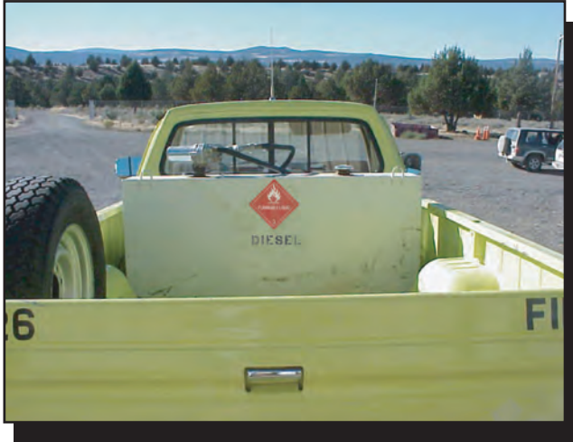
Figure 102—A typical nonspecification tank used for transporting diesel. This photo has been digitally manipulated to show the proper DIESEL marking.
