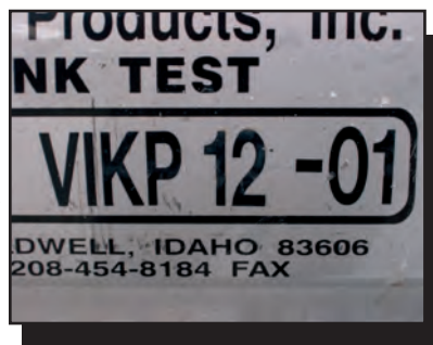
Figure 98—Tank inspection markings on a DOT-406 tank. This tank was last inspected during December 2001.
