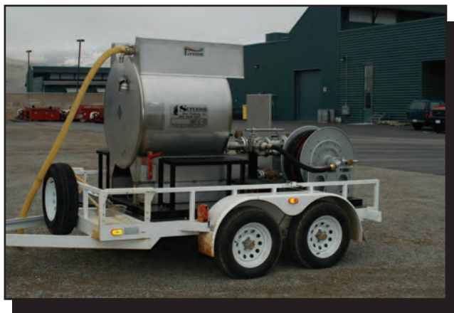
Figure 91—A 240-gallon DOT-406 tank being used to mix gelled fuel.
