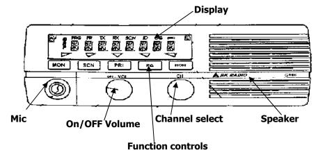
**Mic** – Connection for Mic, keypad on Mic is used to change groups and alter scan lists
