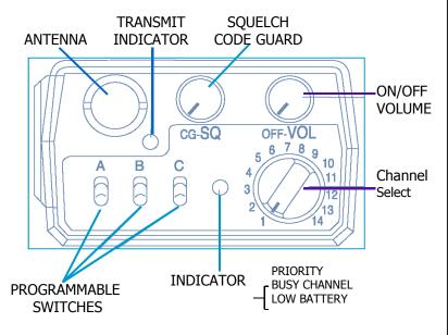
**Antenna** – Antenna connector – it should not turn with antennae **Transmit Indicator** – Red light illuminates when in the transmit mode
