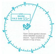
Figure 5-9: Compass Rose Oriented to Magnetic North
