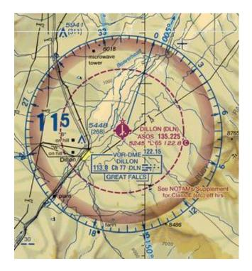
Figure 3-9: Class E Airspace Designated to the Surface by a Dashed Magenta Line
