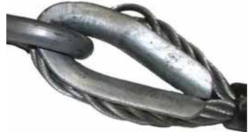
Figure 9. Deformed Thimble and Hook.
