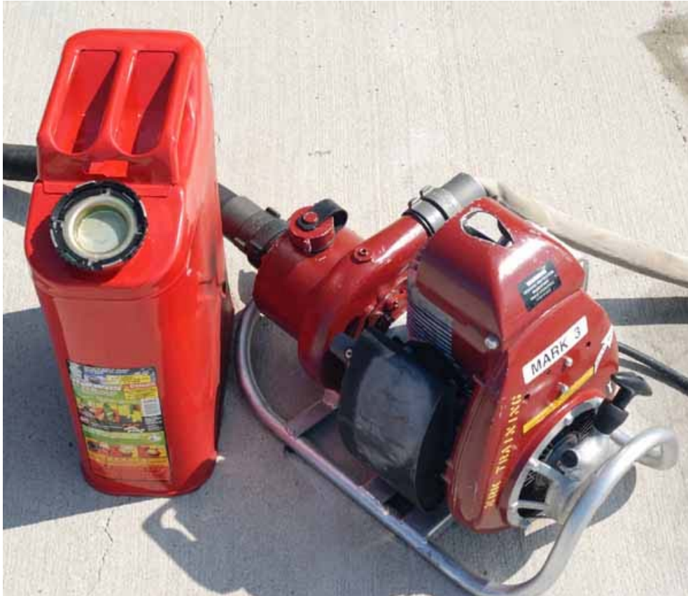
The pump and water can used for testing. Note exhaust soot on side of water can
