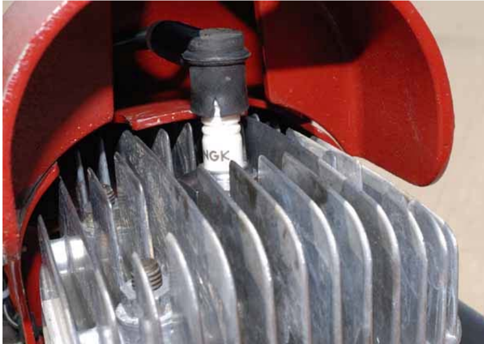
Cracked ignition lead wire boot on Mark 3 pump engine
