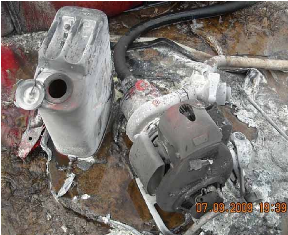
The pump involved in the incident. Note the location of the fuel tank.
