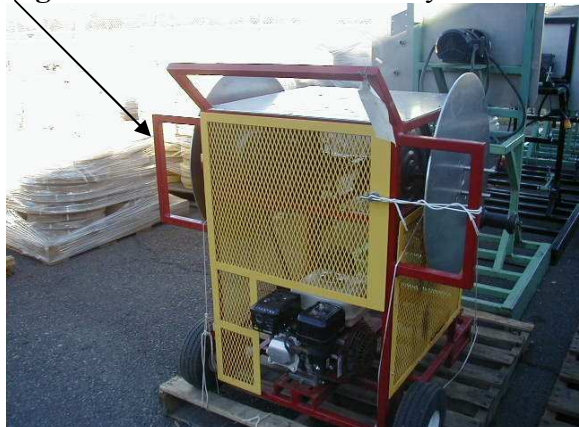
Figure 1. Hose Roller with safety features.
