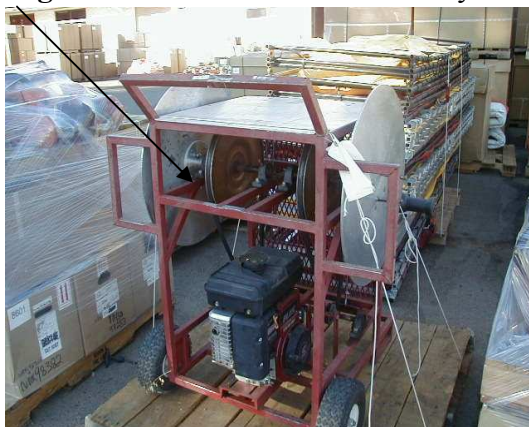
Figure 2. Hose roller without safety features.
