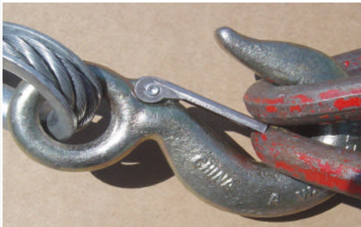
Figure 1 – Lead line hook and cargo net links incompatibility.
