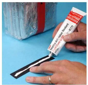
STEP 1: Perform all work in a well ventilated area. Cut the webbing to proper length with a heat knife or sear the ends with a match to prevent them from fraying. Apply a thin bead of adhesive to the nylon webbing.
