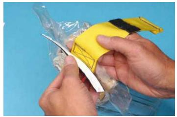
STEP 3: Apply the webbing to one side of the pull strap attachment area and smooth it in place. Repeat on the opposite side of the pull-strap attachment area.
