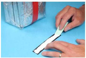
STEP 2: Spread adhesive so it is 1/16 inch thick.
