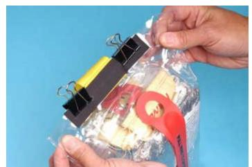
STEP 4: To ensure positive contact until the adhesive cures, use clothespins or paper binders to hold the webbing in place. The adhesive cures in 24 hours.
